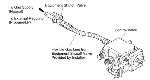
Figure 36 - Attaching Flexible Gas Line To Control Valve
